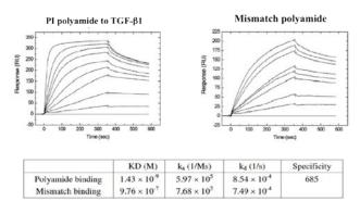
obtained from Biacore assay. Fast binding of polyamide to the target sequence occurred relative to that of mismatch to allow match binding to reach equilibrium at highconcentrations. Specificity of Polyamide to targeting dsDNA is 685 times to Mismatch polyamide (Matsuda et al. 2006).
